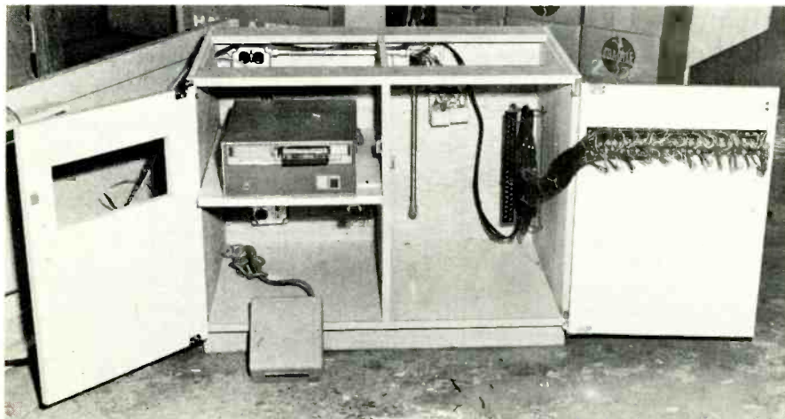
Fig. 4 When desk panels are open, there is easy access to all cables.
